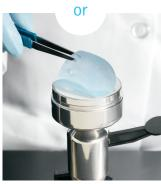
Place the membrane and blue paper on a wet filtration support. When wet, the blue paper curls enabling you to easily remove it using your forceps.
