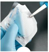
Utilizing sterile forceps, peel back the film and separate the blue paper from the membrane. Remove the membrane with the forceps.
