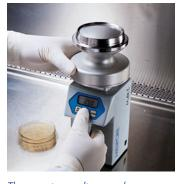
The consistent distance between the sieve and each M Air T cassette ensures reproducible air flow.
