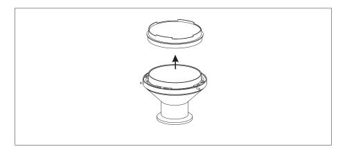
3. Place the sieve, cone adapter and pressure reducer on the cassette and lock it into position.
