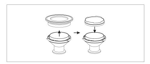
8. Remove the cassette by grasping the "wings" and lifting it off the sampling head.
