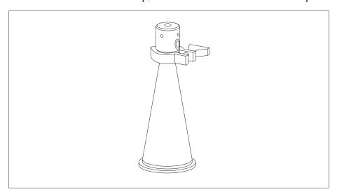
2. With the 4-inch TC clamp, connect the cone adapter to the impaction sieve and then autoclave.
