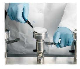
The sealing lip of the Microfil® funnel avoids the risk of membrane by-pass by microorganisms. The clipping (1) holds the funnel firmly on the filtration support. After filtration, the funnel is removed and the membrane is lifted together with the membrane support (2) by simply pressing the lever (3). The membrane can now be conveniently removed from the support using forceps.
