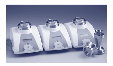
For even greater throughput, a high-volume workstation of up to three Milliflex PLUS pumps can be set up.
