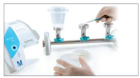
4 Easily remove the membrane after filtration
