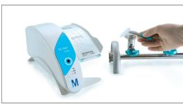
Place the membrane on the EZ-Fit™ Manifold
