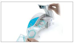
Pull the roll out until the first membrane is visible, then close the cover
