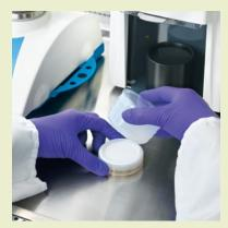
Take the unit out of the MilliSnap system and remove the funnel
