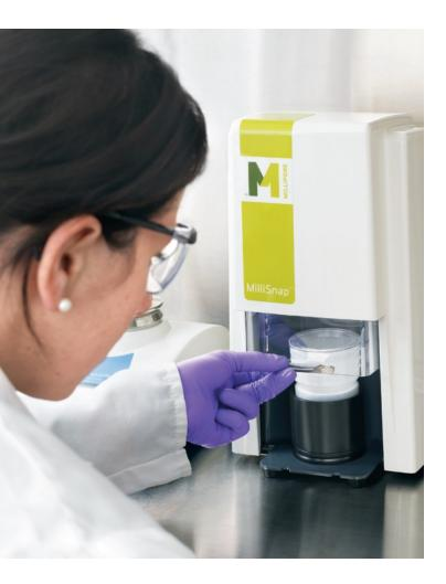
Designed to simplify your workflow, the MilliSnap plug and play system is a hands-free method for separating your Milliflex funnel and attaching the membrane to the Millipore media cassettes. The unique convex shape of the Milliflex membrane combined with the MilliSnap system ensures proper contact between membrane and media.
